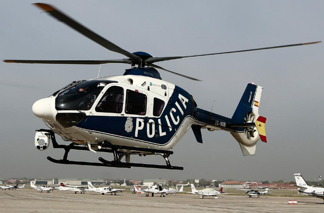
**Objective of this project.** Purchase of two sets of consoles and auxiliary equipment for the installation and operation of the LEO II-A5 and Starsafire HD mission systems from FLIR Systems, and the SkylinkHD image transmission antenna from Troll Systems, on the EC135P2+I helicopter models.
